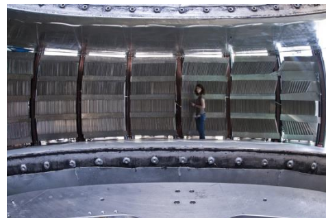
1D detector banks of the spectrometer TOFTOF at MLZ. Image credit to Jürgen Neuhaus.
